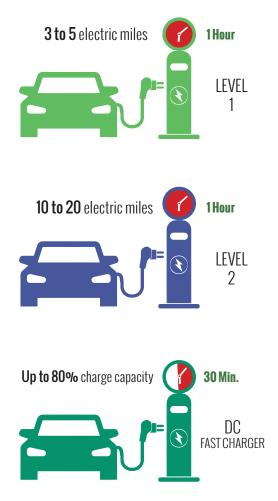
**Level 1 charging:** Provides the slowest charge, around 3 to 5 electric miles per hour. Even at this slow speed, however, the majority of electric vehicle owners plug in at home to refuel.
